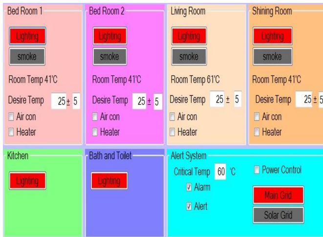
Fig.11. Screenshot of Graphical interface of Smart home temperature control (Abnormal State).
